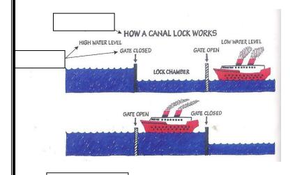
Engineers can raise the water level inside the lock chamber to the higher water level or lower it to the lower water level to allow ships to pass.
