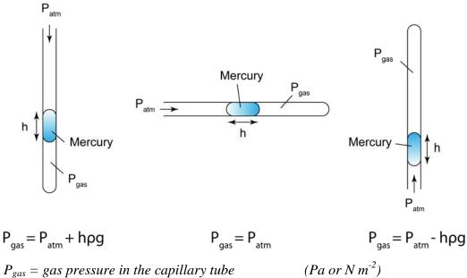
$P_{gas} = gas \ pressure \ in \ the \ capillary \ tube$   $P_{atm} = atmospheric \ pressure$   $h = length \ of \ the \ captured \ mercury$   $\rho = density \ of \ mercury$  $g = gravitational \ field \ strength$
